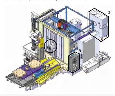
1. Flushing system to remove chips from the spindle top and slide cover.
