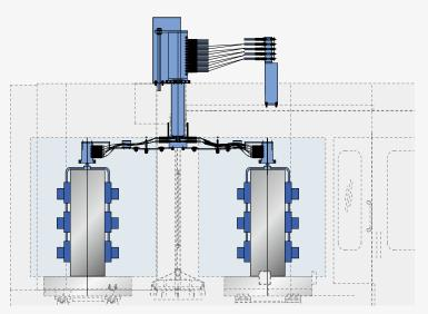
The overhead connecting system allows pallet change and table index cycles whilst maintaining hydraulic/pneumatic connections to fixtures .
