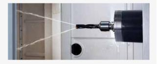
Spindle-through coolant spray device option
