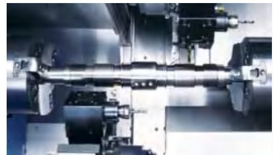
Different cutting processes can be carried out on a single work piece with the upper and lower turrets simultaneously.
