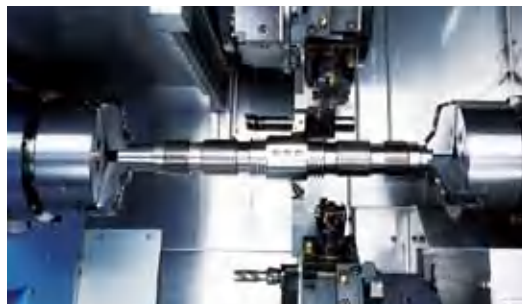
Turning at the same position is carried out with the upper and lower turrets simultaneously.
